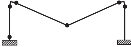
FIGURE 6.28. Feasible collapse mechanism.
